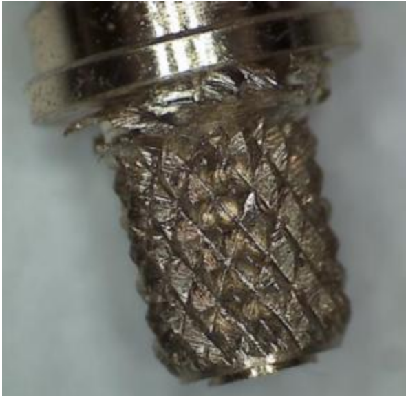
Figure 5-7: Knurl made from CuZn42 with sharp edges and broken material
