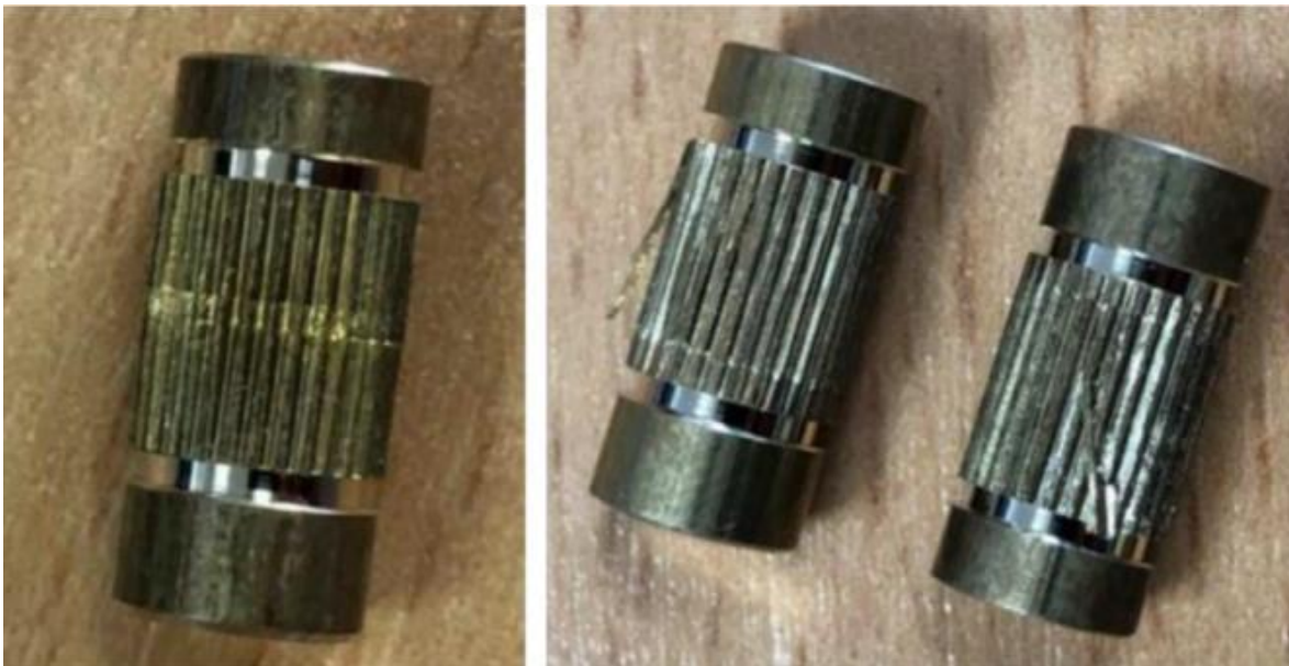
Figure 5-8: Knurl pressed on a component made of CuZn39Pb3 (left) and two knurls pressed on CuZn21Si3P* with loose particles (right)
