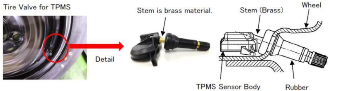
Figure 5-9: Tire valve with TPMS produced from leaded (C3604) and unleaded brass (BZ-5U) after rubber adhesion test
