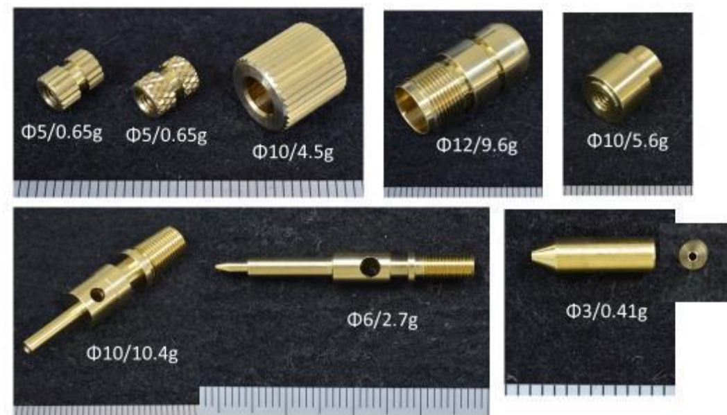
Figure 5-15: Machining small-diameter Rods [rod diameter (mm)/component weight]
