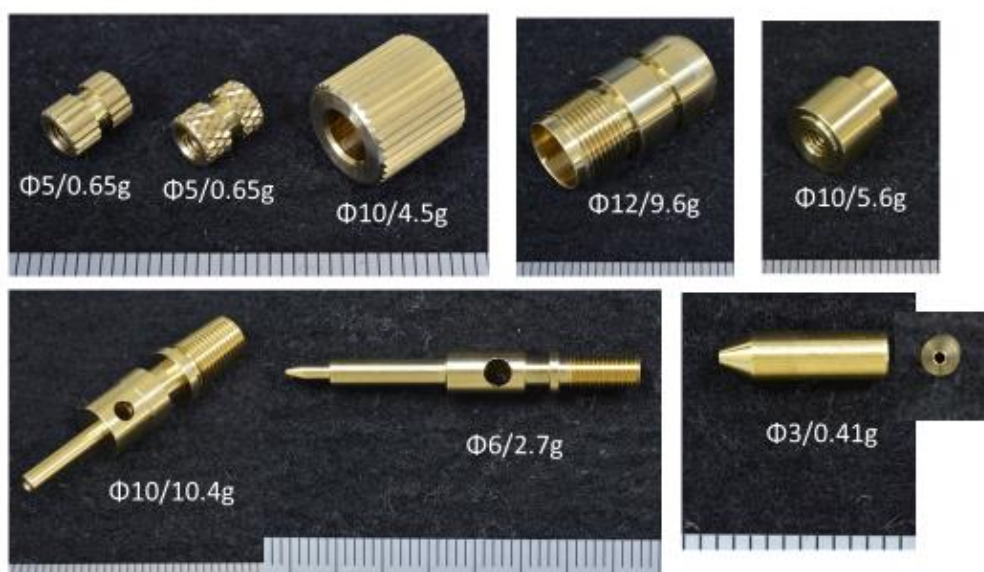
Fig. 7: Machining Example 1 – Machining Small-Diameter Rods for Production of Parts Assumed to Be Used As Auto Parts or Electrical/Electronic Parts [rod diameter / component weight]
