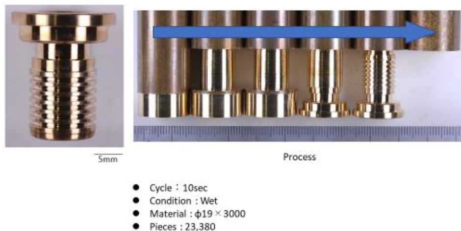
Fig. 8: Machining Example 2 – Machining with Automatic 6-Spindle Lathe
